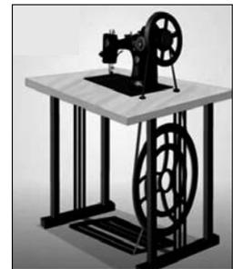
We see even we stop supply of driving force to the bigger wheel it still continues to run for a short time because of its moment of inertia.
